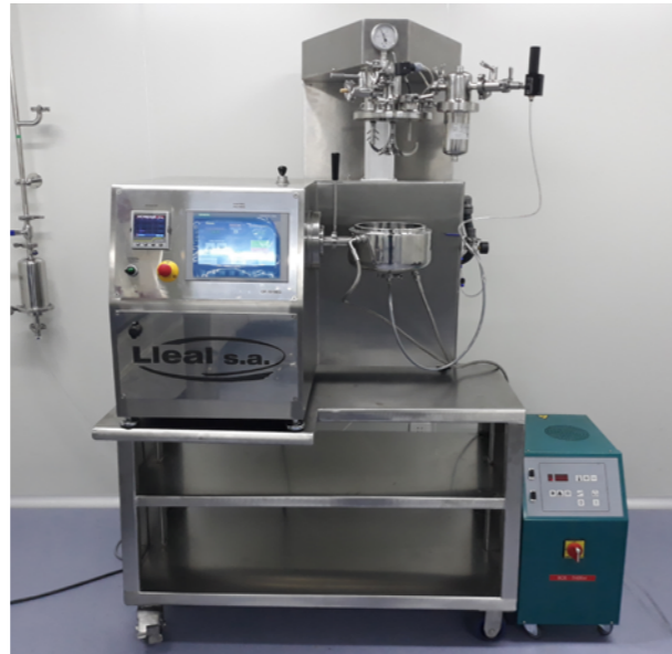
MGR-1 TRI-CHOP granulator installed in a cleanroom.
