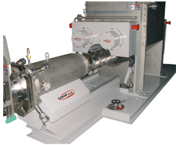
View of disassembling an extruder screw for cleaning
