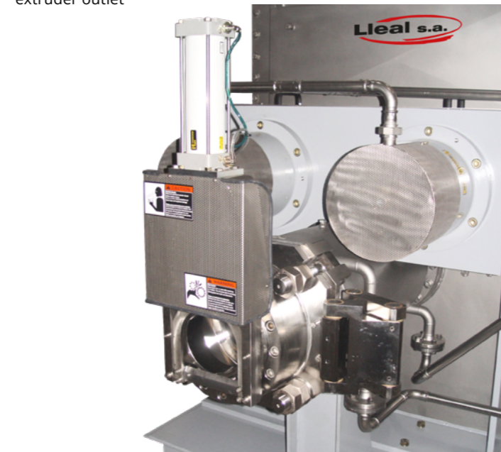
Pneumatic cutting guillotine at extruder outlet
