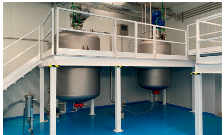
Plant for the production of hydro-alcoholic gels: 2,000 L reactor for manufacturing and a 2,500 L formulation adjustment tank.
