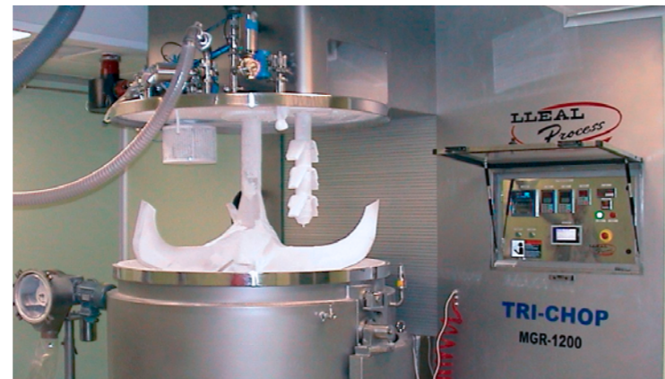
View of a MGR-1200 TRI-CHOP with panellised bedplate, installed in a clean room of a pharmaceutical company
