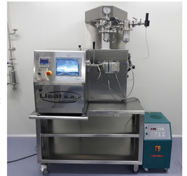
MGR-1 TRI-CHOP granulator installed in a clean room
