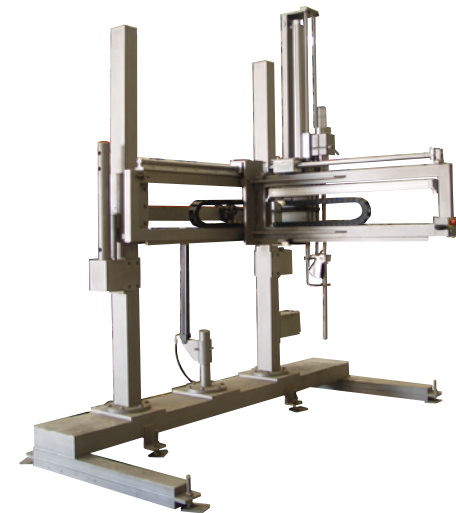
PEN-2000-C packaging machine, fully made of stainless steel with Cartesian translation system
