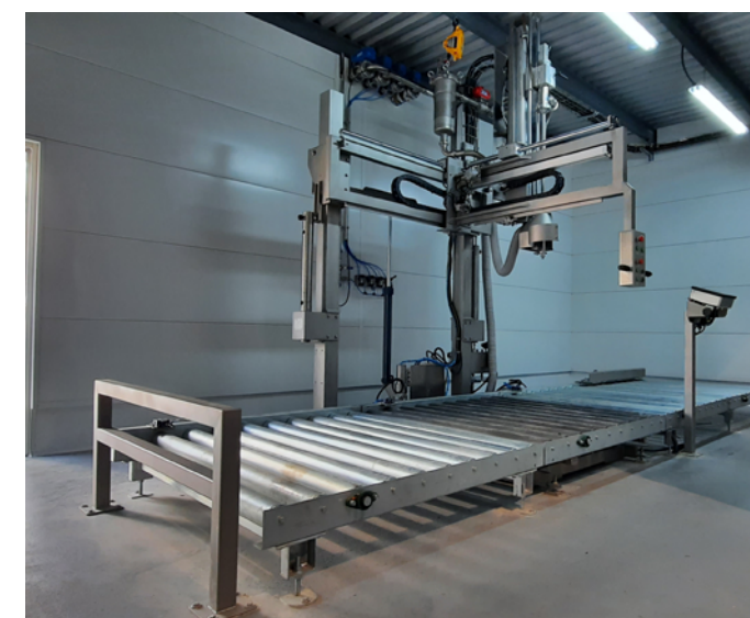
PEN-2000-C packaging machine equipped with motorized roller conveyor for the infeed and outfeed of the containers.
