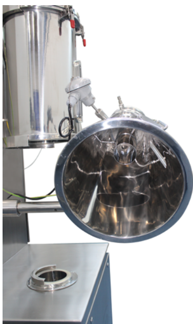
Detail of the Wurster tube installed in the product hopper, in the discharge position.
