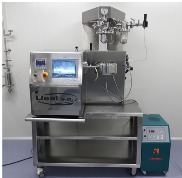
MGR-1 TRI-CHOP granulator installed in a cleanroom.
