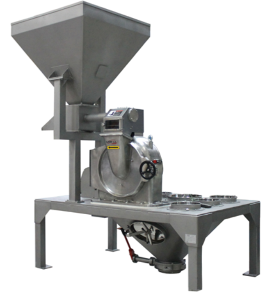
Grinding plant K-500-B, with TK endless screw feeder equipped with special 600 L hopper. Discharge by means of manually operated butterfly valve.
