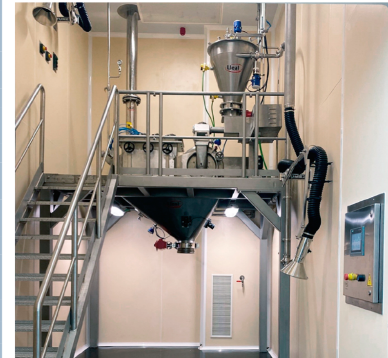
K-315-MO grinding installation, prepared to work in ATEX zone. The equipment is fed by a TS-VAC 50 pneumatic conveying system.
