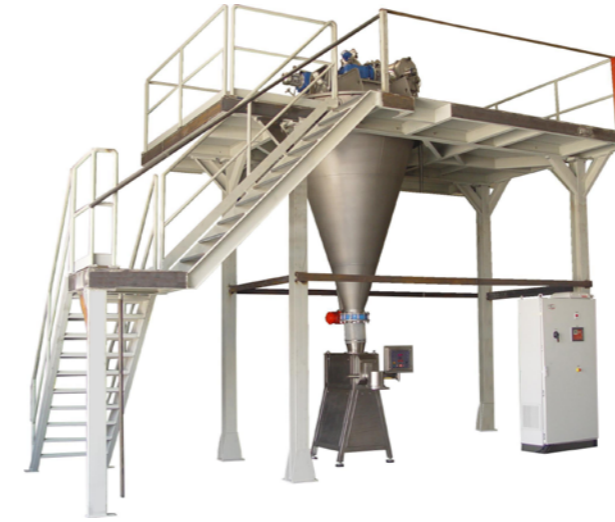
C-1000 mixer assembled on a structure, fed by a centrifugal sieve CEN-450 and coupled with a bagging machine S-50-T for unloading.
