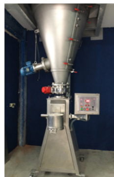
C-500 mixer with intensifier assembled on the lower side. It features a lateral gate for easy cleaning.
