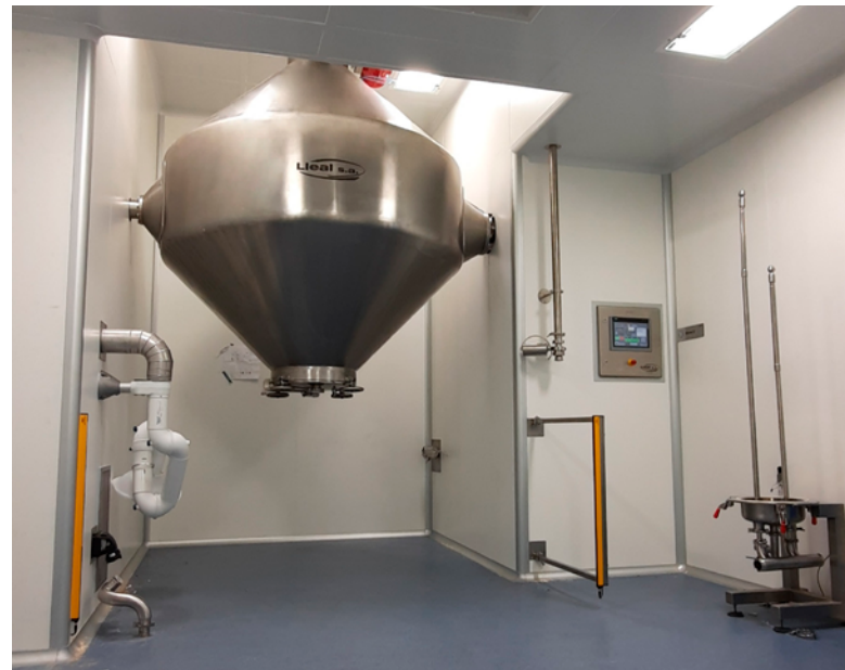
BC-4200 biconical mixer, designed for the manufacture of pharmaceutical products and installed in a clean room.
