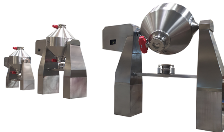
View of three bi-conical mixers models BC-1000 and BC-600, with pneumatic valves mounted on the two mixer mouths and extendable bellows for product discharge.
