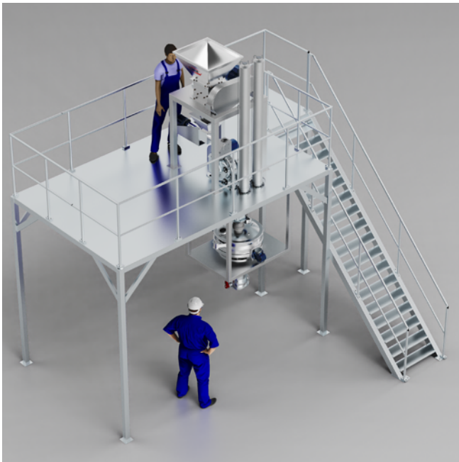
Cascade plant consisting of an ST-315 crushing mill, a Komodin mill and a vibrating sieve shaker.
