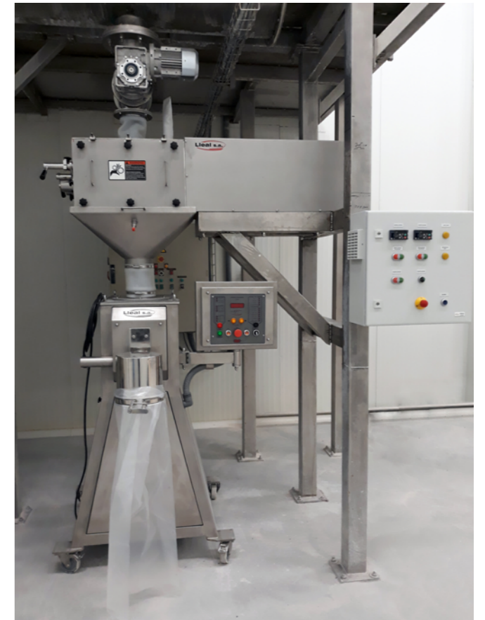
S-50-T bagging machine with open-bags head, fed by a CT-400 Geminis granulator
