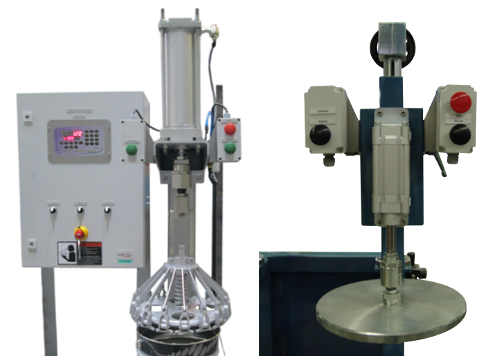
Pail lid crimping device and metal disc for pressure closure
