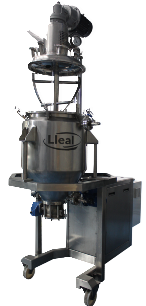
MVH-100 helical mixer with double jacket prepared to work at a temperature of 300 °C. The equipment has a mobile service bench.
