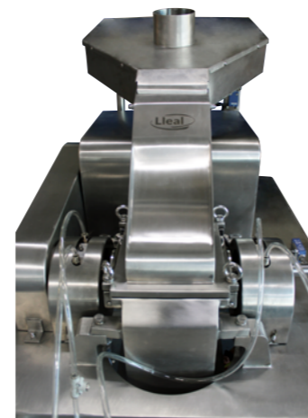
Power supply system prepared for connection to pneumatic conveyor
