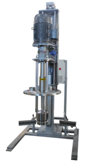
MI-10/M immersion mill with fixed wall support. Pneumatically operated head-cover lifting system.
