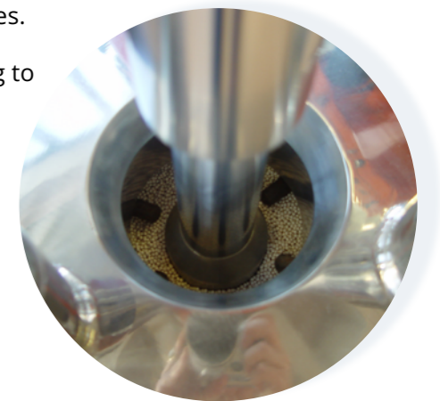
Detail view of the interior of the basket milling loaded with zirconium balls.
