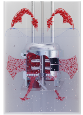
Operation diagram of a basket mill.
