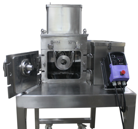
View of the interior of an MG granulator
