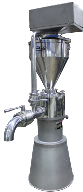
MCV-4 mill with recirculation system and 50 L hopper equipped with an anchor-type agitator.
