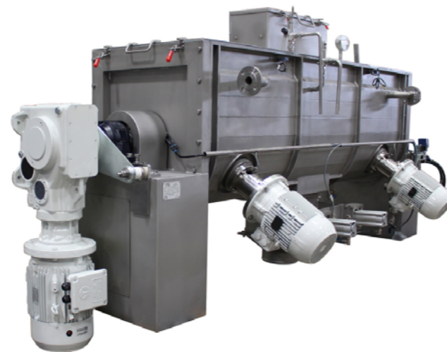
MB-1500 CTAI ribbon blender with double jacket for heating/cooling and lump-breaking turbines assembled at the bottom. Equipment for the manufacture of food additives.
