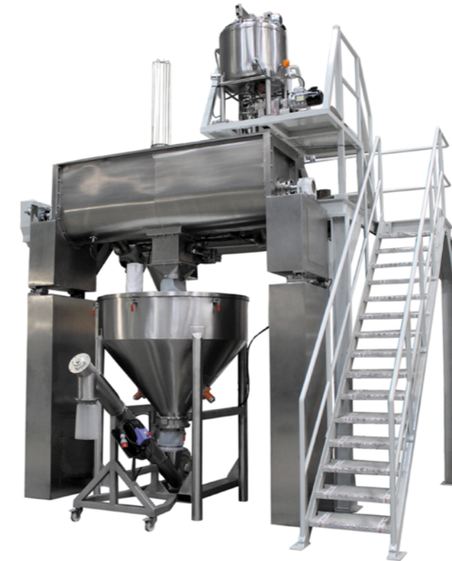
Mixing installation consisting of a fusing kettle on the upper part, discharging hot syrup onto the MB-700 ribbon blender. Equipment for the food industry.
