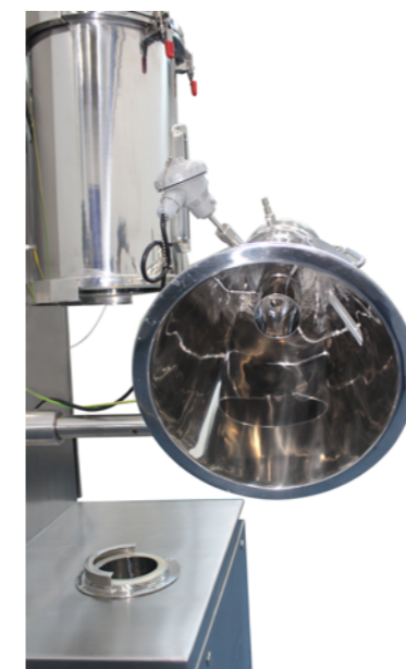
Detail of the Wurster tube installed in the product hopper, in unloading position.
