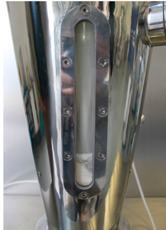
Detail of the product hopper. The fluidising product is visible through the sight glass
