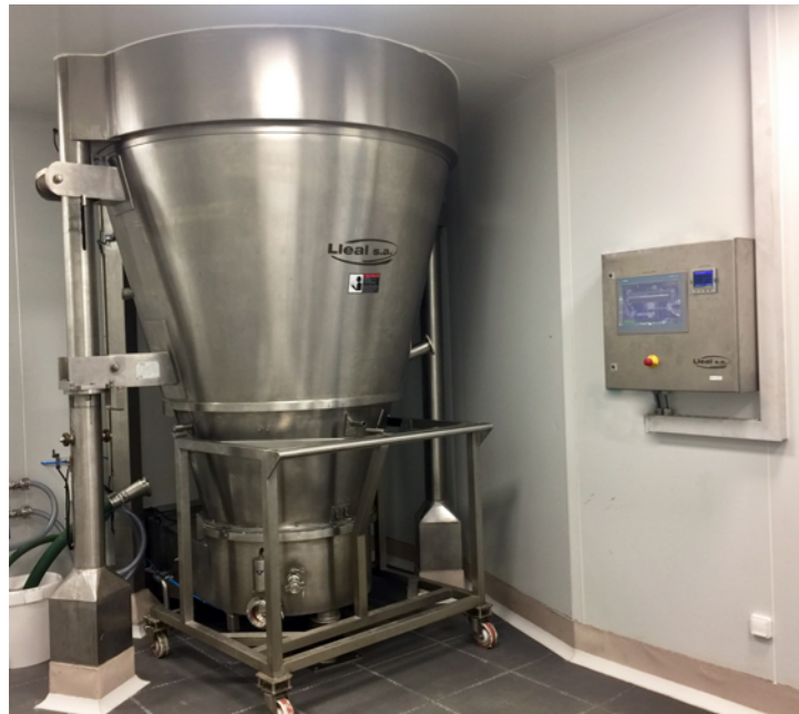
High-flow fluid bed, in special execution, with internal rotating plate, installed in the customer's facility.
