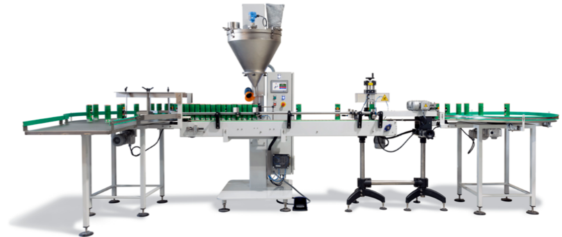
Powder filling line for powder in cans, with dynamic operation and volumetric dosing control, installed with feeding rotary table for containers and collection table at the end of the line.
