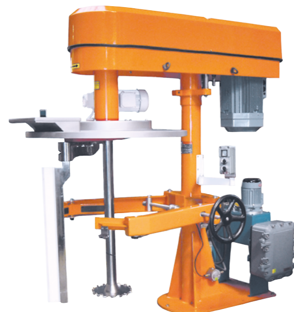
Coaxial dissolver of 18,5 kW with clamping arms and jaws. Atmospheric lid.
