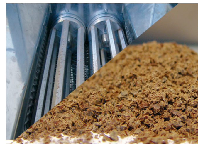
Detail of the granulating rollers of a CT-400 with mesh at the bottom and detail of the resulting product.
