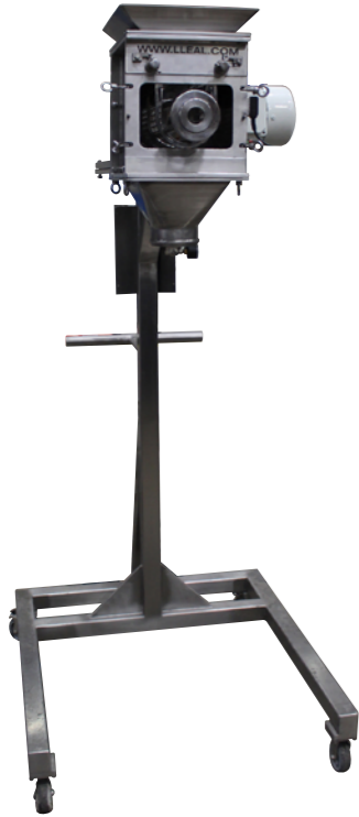
CT-150 granulator with the front door removed, allowing to see the rotor, slightly pulled out of the chamber
